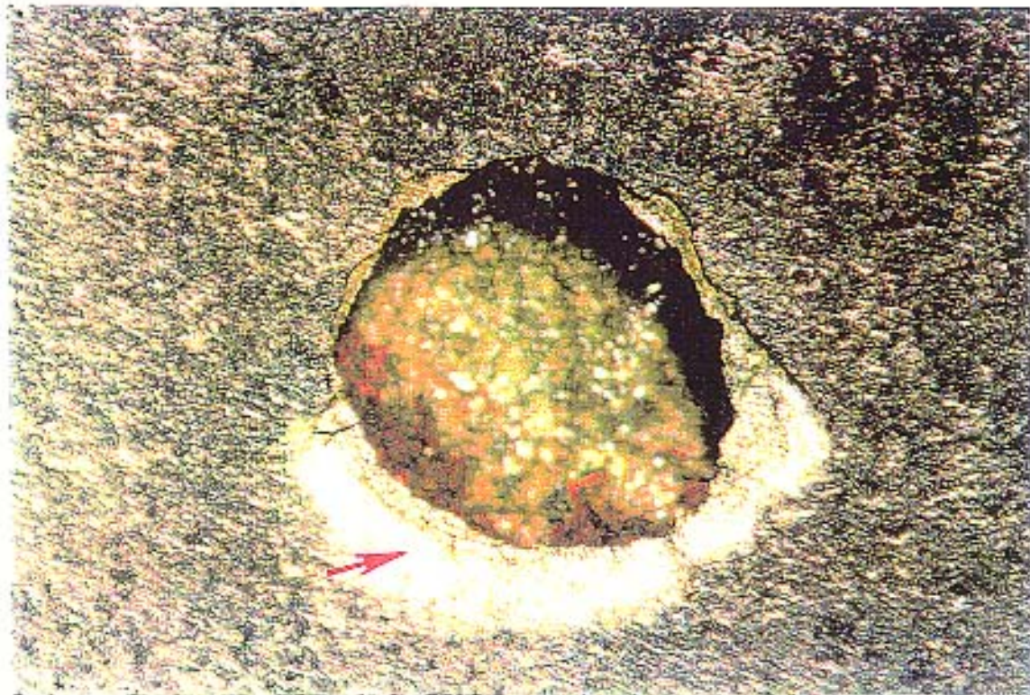
Figure 3 Closeup of Pit Under Holiday in Water Phase Magnification: 30X
